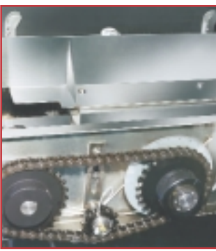
⑤ "Phaser" adjustment allows easy changes to compression pocket size for optimum squareness of trays.
