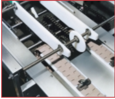
② Positive tray transport keeps control of tray during transfer from magazine.
